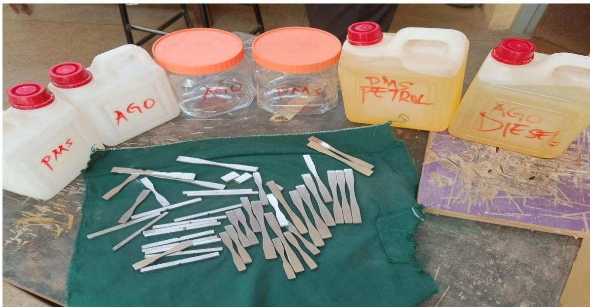
Figure 3.2: Prepared carbon steel coupons after grinding, polishing and degreasing before weighing
