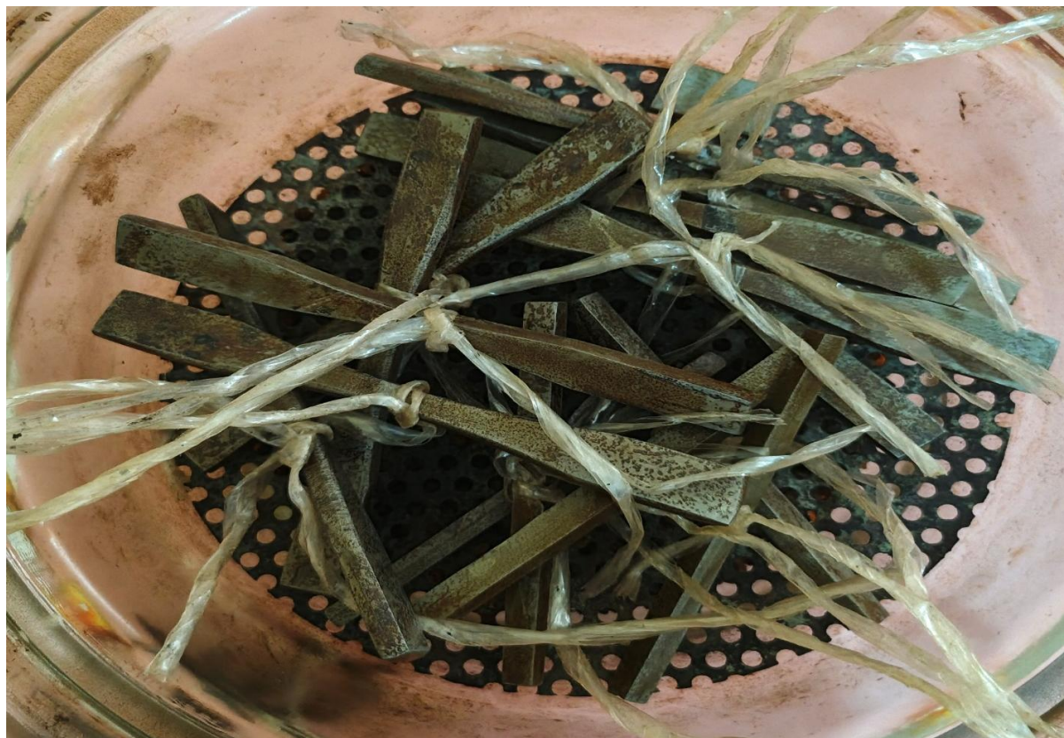
Figure 3.4: Corroded specimens after HCl cleaning, distilled-water/ethanol rinse and desiccator drying, immediately before final weight measurement on the analytical balance
