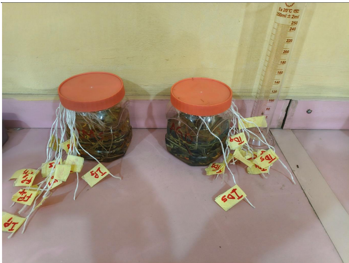
Figure 3.2: Sealed plastic containers with carbon steel coupons immersed in PMS and AGO
