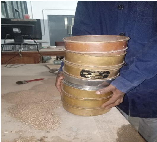
Plate V(a): Fine aggregate grading
