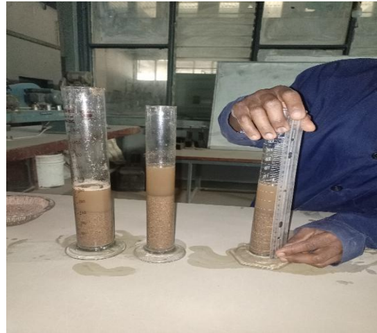
Plate V(b): Silt and clay content of sand
