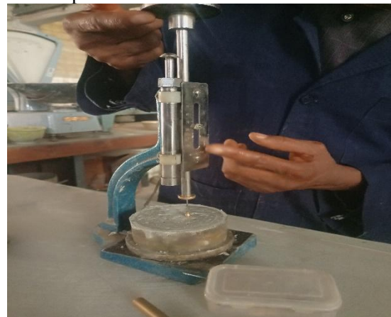
Plate IV: Final setting time test of cement
