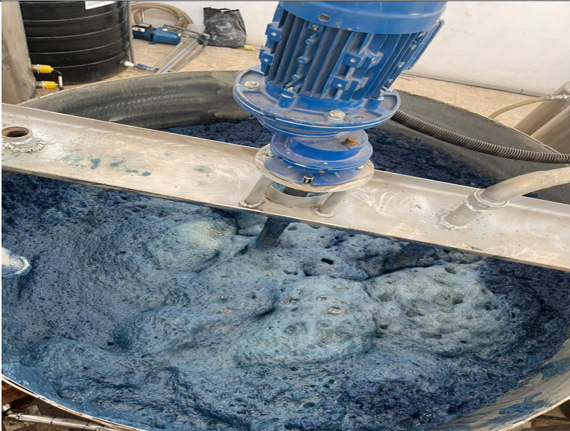
Figure B3: Oxidation of fermented broth in the oxidation tank
