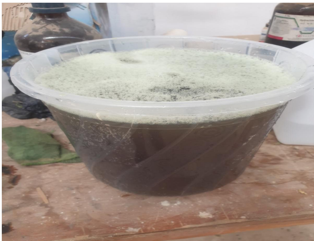
Figure A4: Residual fermented broth after oxidation in batch experiments
