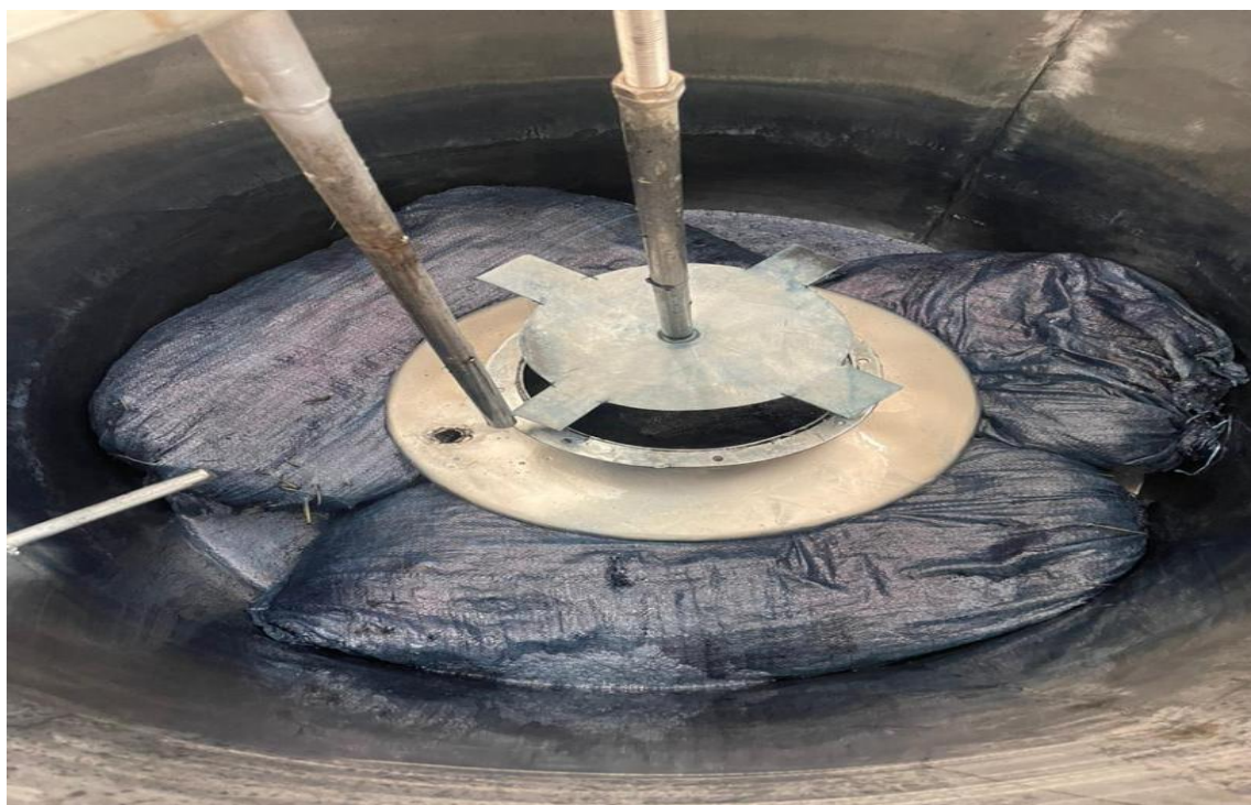
Figure B2: Steeping/fermentation of plant biomass in the steeping tank
