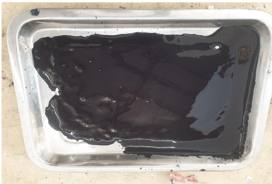
Figure A5: Indigo slurry drying on a tray
