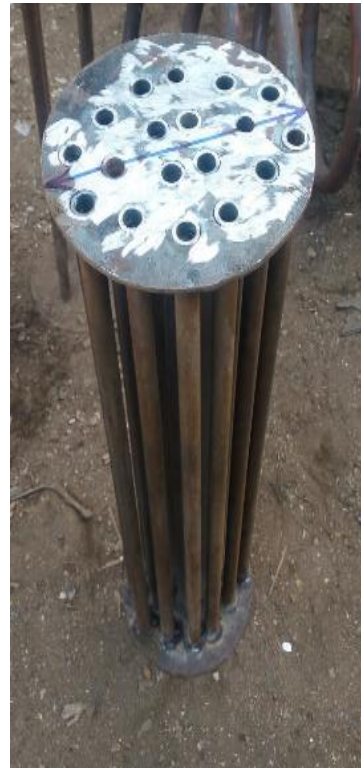
Plate 3b: Heat Exchanger tube
