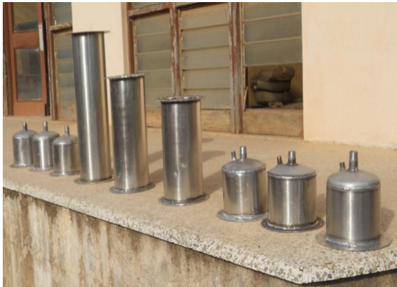
Plate 1a : Parts of the three Fabricated Reactors
