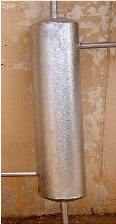
Plate 3a: Heat Exchanger bundles
