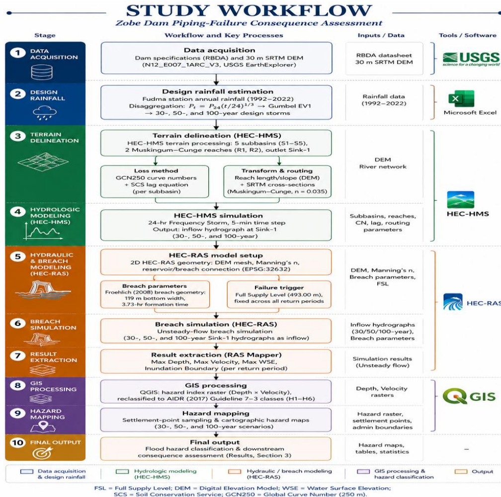
Figure 1: Overall study workflow, from data acquisition through terrain-based HEC-HMS delineation and design-storm hydrograph generation, HEC-RAS breach and unsteady-flow simulation, to GIS-based flood hazard classification.
