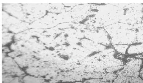
Plate 4: OM Micrograph of As-Cast Al-Si-Mg Alloy (Control)
