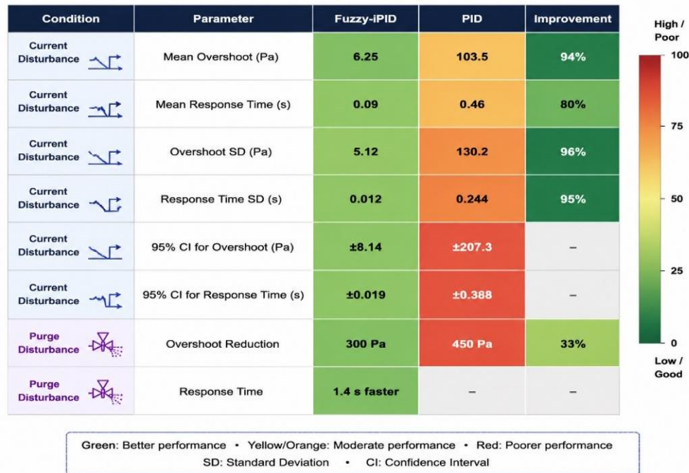
Figure 5: HIL performance comparison of the Fuzzy-iPID and conventional PID controllers under current and purge disturbances.
