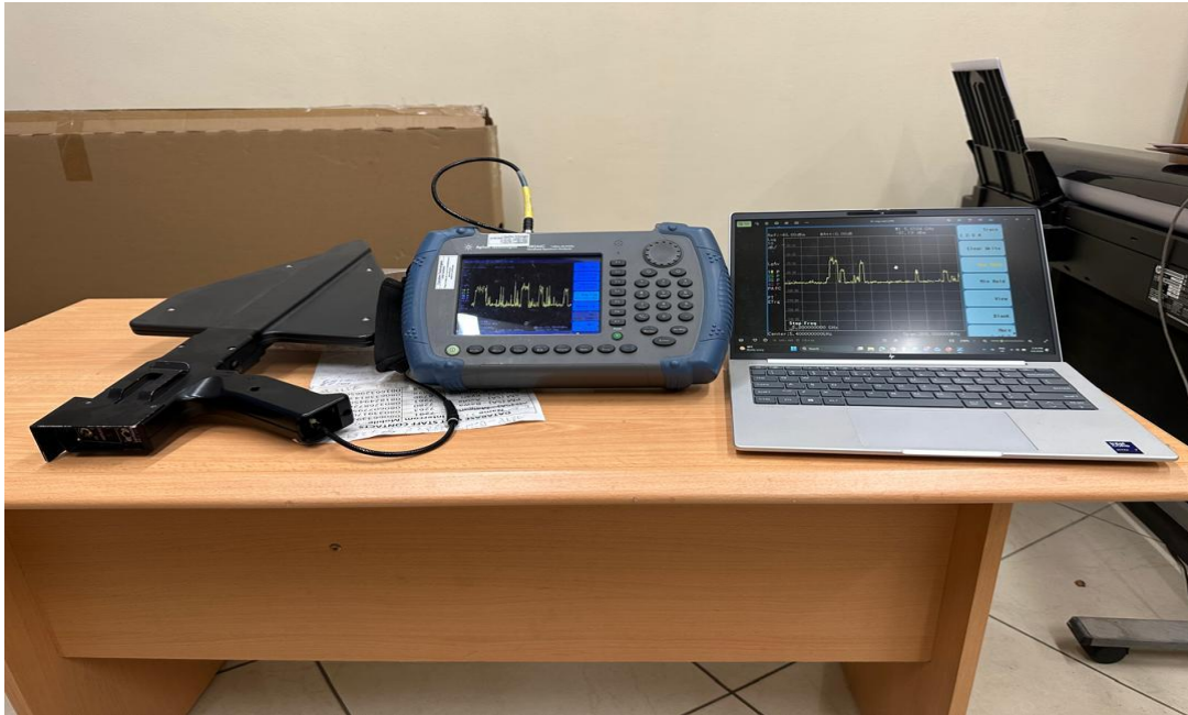
Figure 3: Showing the Spectrum Analyser measurement set-up
