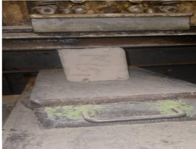
Figure 2: Compressive Strength Test
