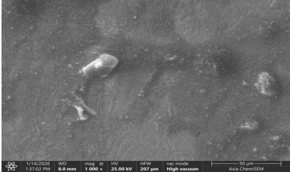
Plate VI: SEM micrograph of austempered sample, Run 5, at 1000×
