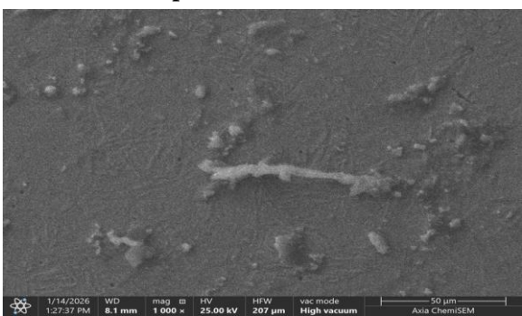
Plate VI: SEM micrograph of austempered sample, Run 5, at 1000×
