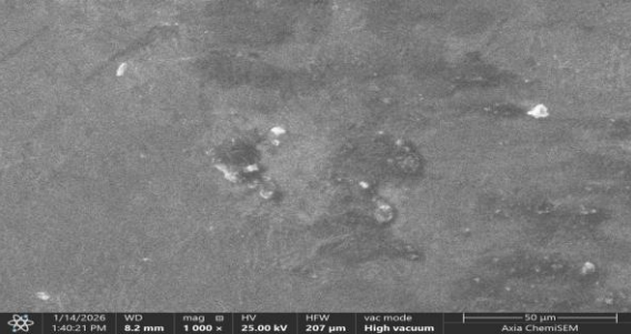
Plate VII: SEM micrograph of austempered sample, Run 6, at 1000×
