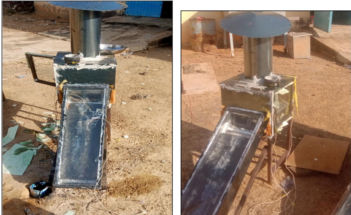
Plate I. The constructed solar dryers.
