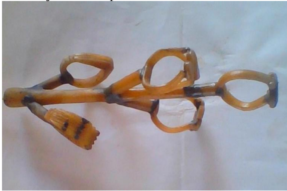
Figure 1: Beeswax Pattern Tree and Completed Investment Casting Mould Prior to Firing.
