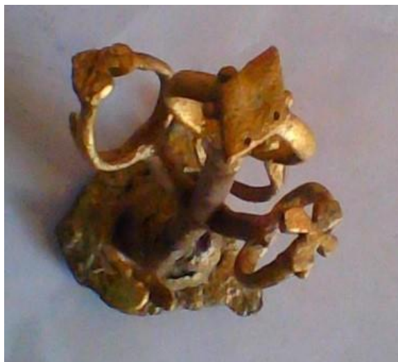
Figure 9: Brass Jewellery Casting Produced from the Investment Casting Mould.
