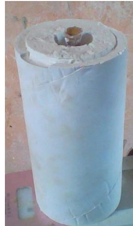
Figure 1: Beeswax Pattern Tree and Completed Investment Casting Mould Prior to Firing.
