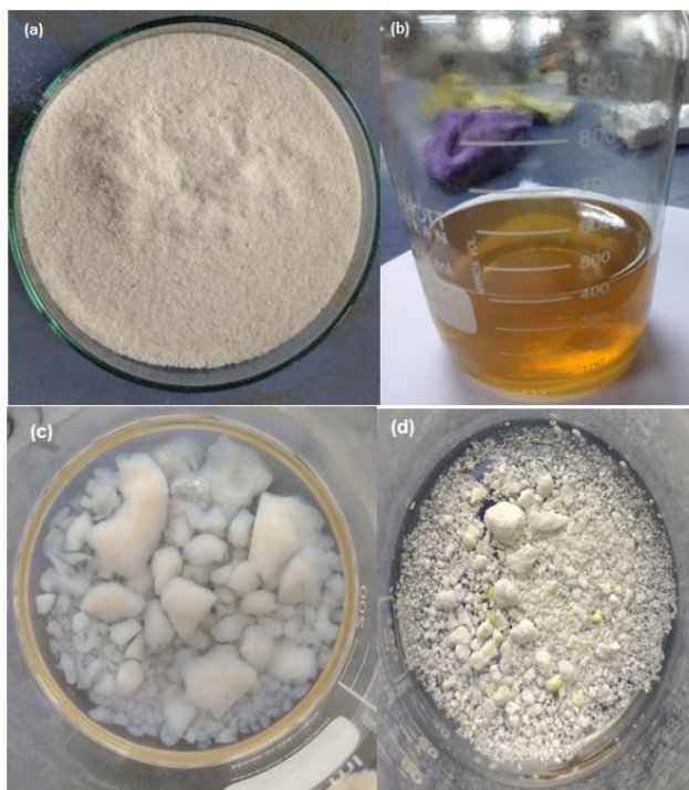
Figure 2: Visual transformation during silica aerogel synthesis: (a) rice husk ash; (b) sodium silicate solution; (c) gel particles in ethanol for exchange of pore water with ethanol; (d) Dried silica aerogel particles.
