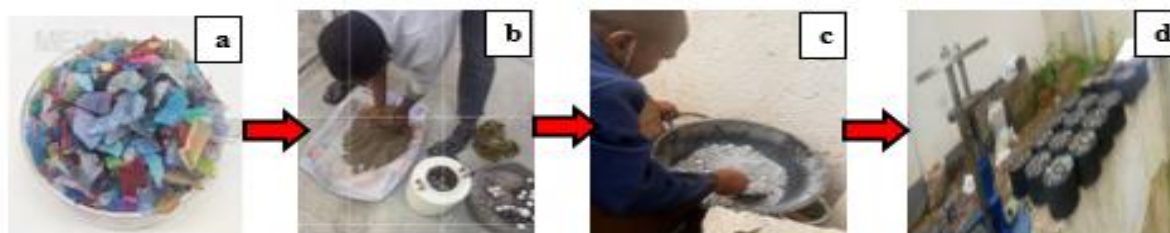
Plate I: Processing of polycarbonate waste (a) pellet polycarbonate (b) pulverized polycarbonate (c) dry mixing of polycarbonate (d) asphalt concrete admixed with polycarbonate
