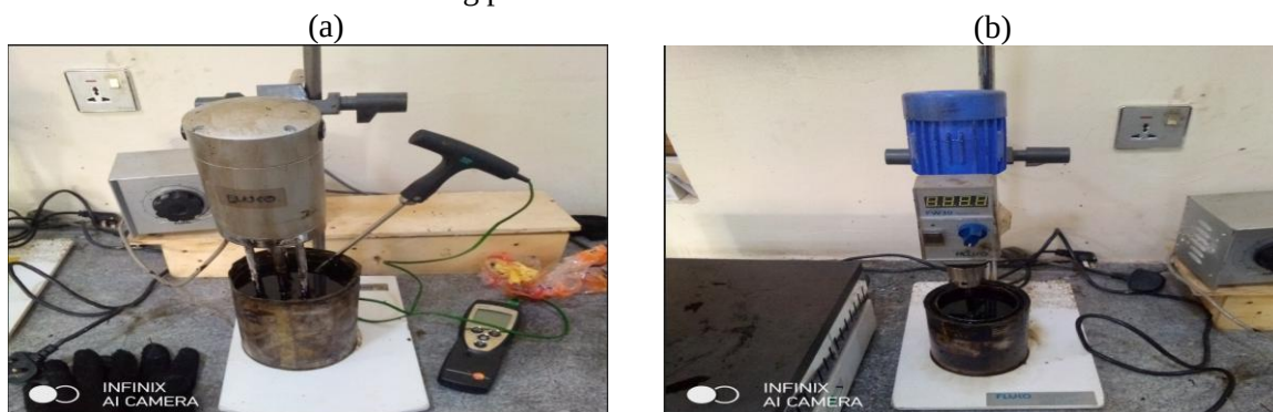
Plate II: Production of metakaolin-based geopolymer modified asphalt binder (a) high shear mixing (b) low shear mixing
