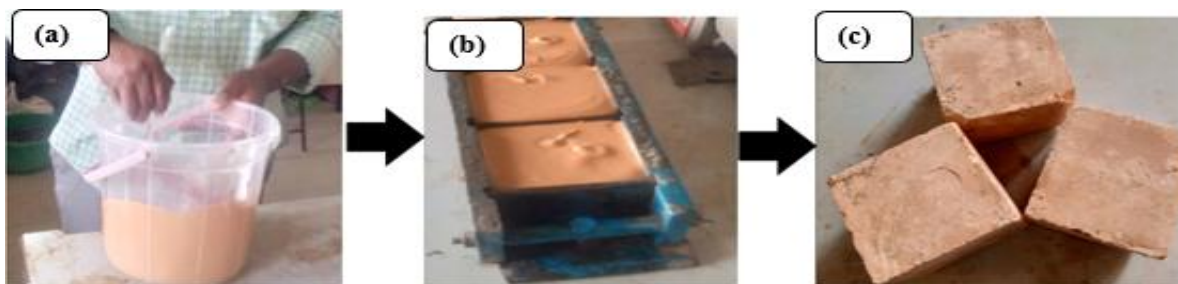
Plate I: Geopolymerisation process: (a) mixing at room temperatures (b) geopolymer paste (c) geopolymer cubes
