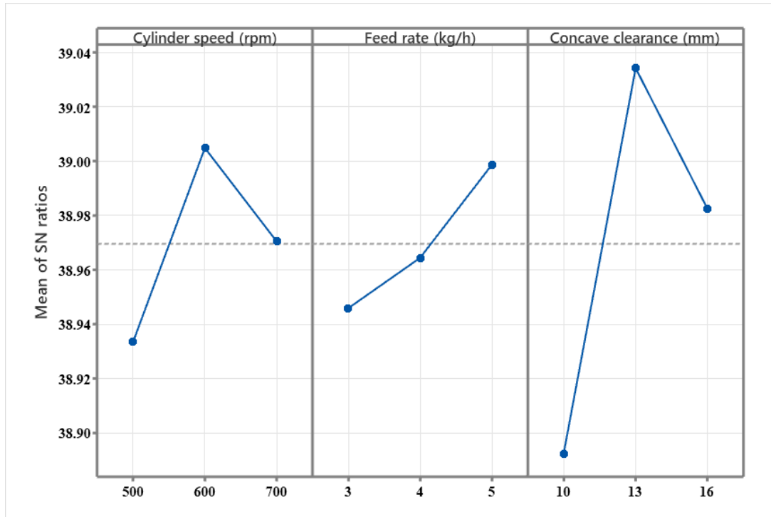
Figure 3: Main effects plot for signal-to-noise ratio (TE)
