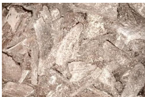
Figure 2: Palm kernel shell (Carbonized charcoal) Sourced at Metallurgy Foundry Laboratory A.B.U Zaria
