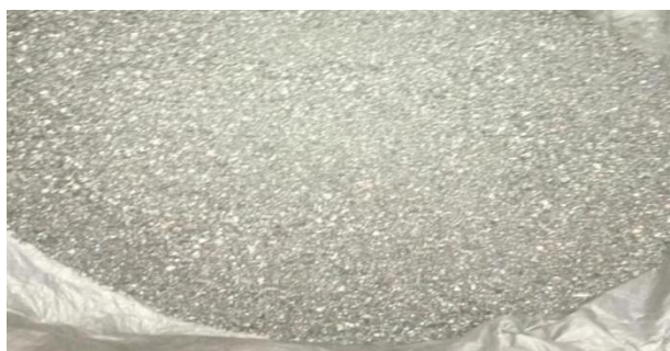
Figure 3: The Grinded Palm kernel shell charcoal (Activated Charcoal). Sourced at metallurgy foundry laboratory A.B.U. Zaria.
